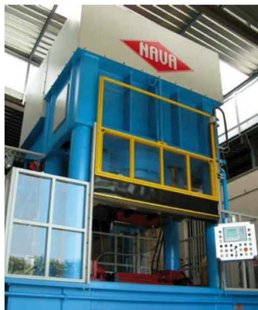
F.lli Nava's 8,000 kN hydraulic press, developed for closing the upper half of the mould with vertical movement, of a pressure multiplier unit
