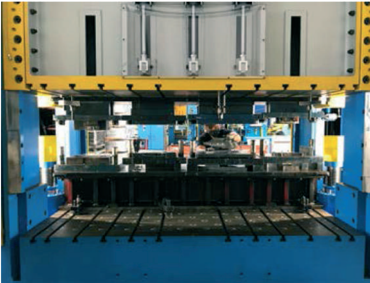
The new F.lli Nava hydraulic press is able to deliver 450 tons of force, in addition to having a 200-ton blank-holder, that consists in a single table with 4 adjustment points freely programmable electronically
