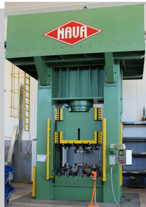
5,000 kN hydraulic press, with 1,600 x 1,000 mm plates, with three totally independent "third effect" moulding functions and differentiated blank-holder
