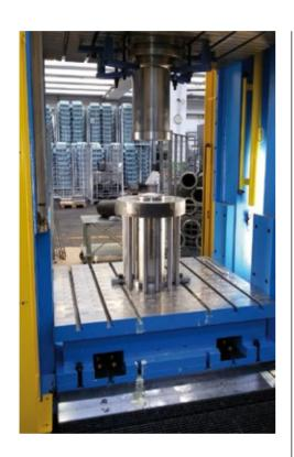
NAVA company is proud to present presses featuring conventional drawing and active downward drawing. The top of the range model is 2MI 1100/500 for drawing, with 11,000 kN maximum hammer force, 5,000 kN bottom sheet press, 800 kN third top effect, and 2,500×1,800 mm processing shelves. The model with lesser force is 2MI 500/300 for drawing, with 5,000 kN maximum hammer force, 3,000 kN bottom sheet press, and 2,500×1,800
